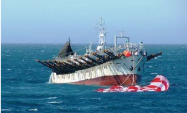
Fig 29. Squid jigger deploying sea anchor, with jigging machines ready for fishing.
