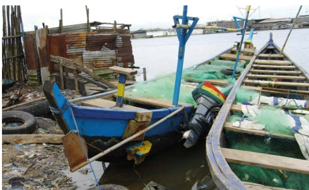
Fig 26. Typical West African drift net canoe, about 12 m in length. Note the lack of lights, fishing signals
