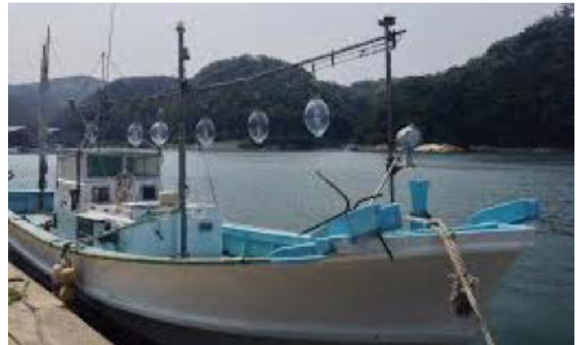
Fig 31. A typical inshore squid jigger. Note the lights for attracting squid.
