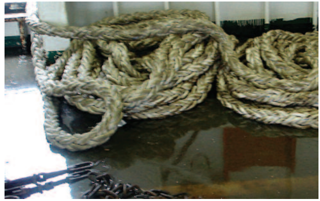
Ropes badly stored on wet deck
