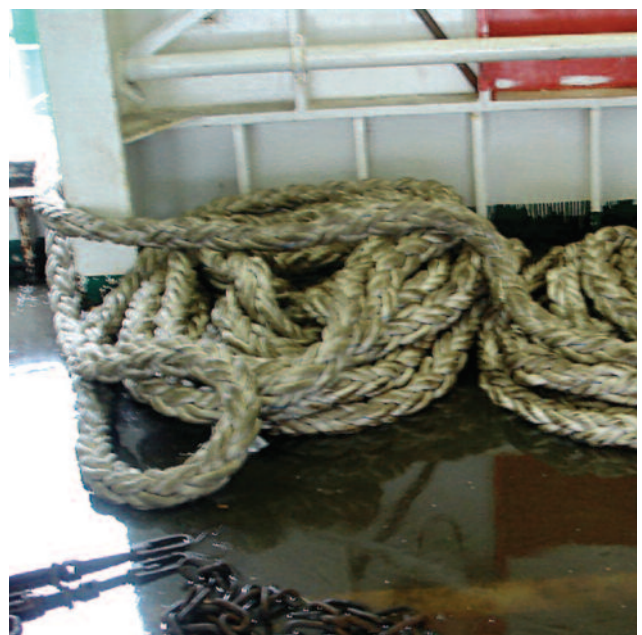
Ropes badly stored on wet deck
