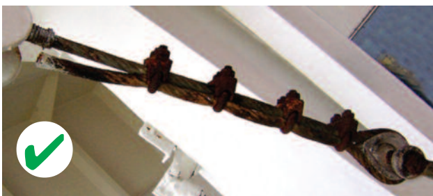
Once ropes have been hauled tight they should be secured to bitts as in the good example on the left
