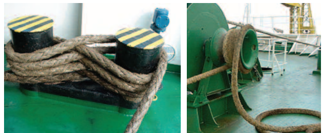
Once ropes have been hauled tight they should be secured to bitts as in the good example on the left
