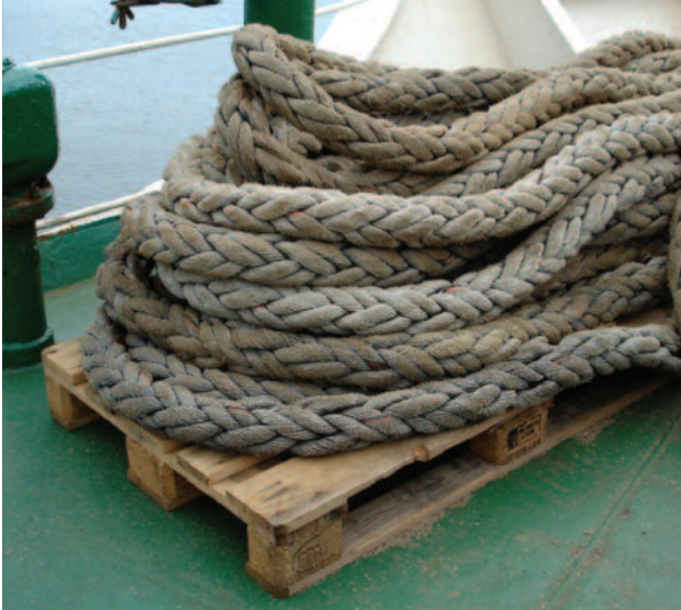
Ropes correctly stowed off deck
