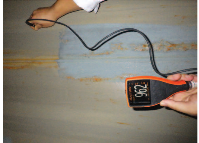
Measuring the dry film thickness (dft)
