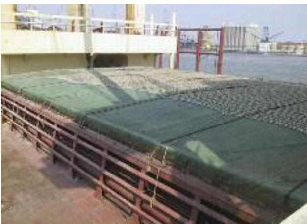
Tarpaulin type hatch covers, properly battened down and ready for going to sea
