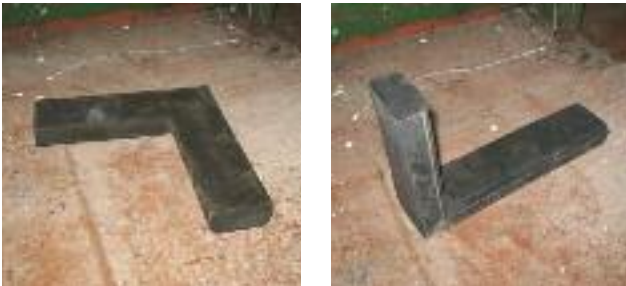
Different shapes of packing rubbers (from left to right: linear rubber, end piece with solid nosing, flat corner and vertical corner)
