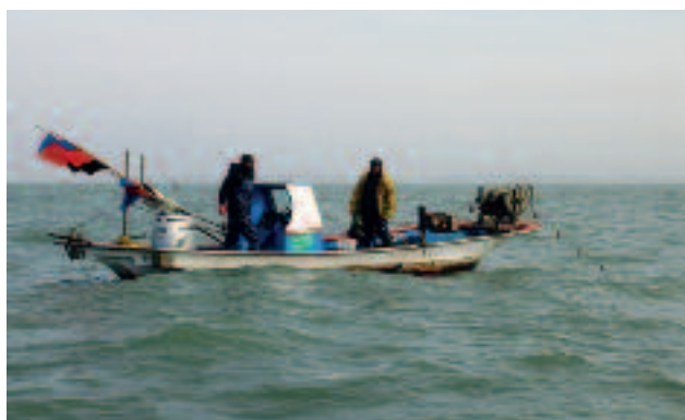
Fig 3. Small static gear vessel, South Korea. Note the absence of any lights or day shapes.
