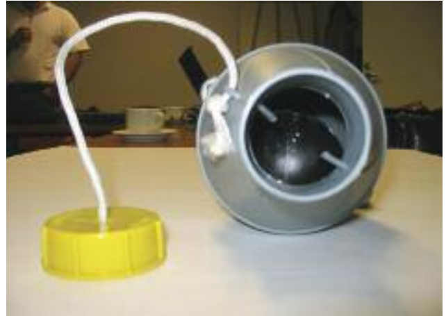
Drain valve with ball inside acting as non-return system
