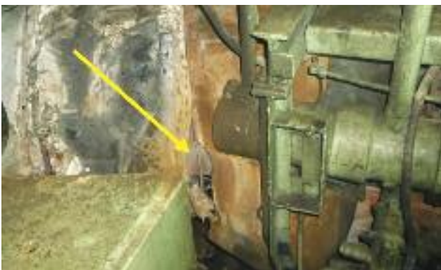
Small portion of exhaust surface exposed (as arrowed)
