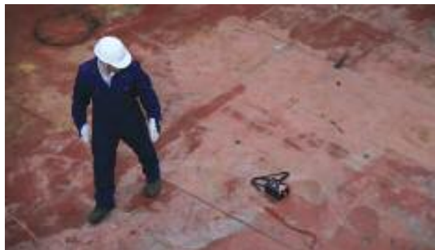
Transmitter being placed in the ship's hold
