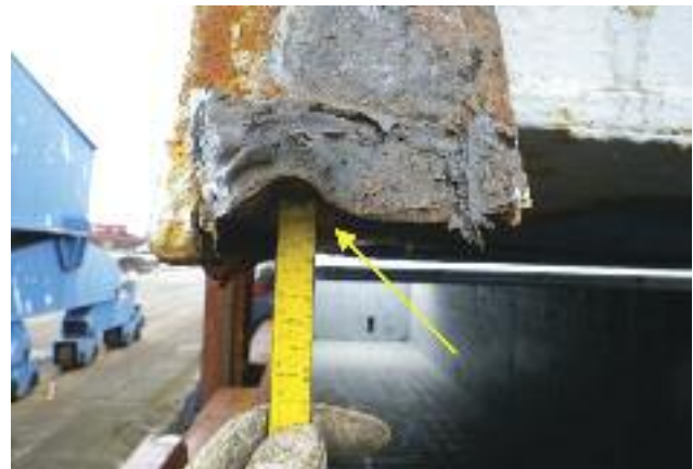
Deep permanent groove in packing rubber as a result of overcompression. Also note the off-centre permanent imprint
