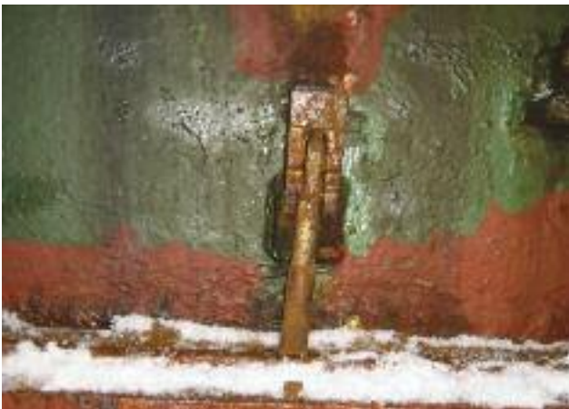
Crooked quick acting cleat (improper vertical alignment)
