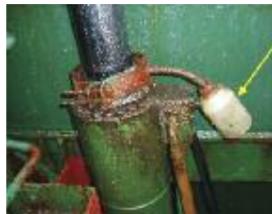
Temporary repair (rubber patch and jubilee clip) and shipboard made systems to contain hydraulic oil leakage from hydraulic piping and cylinders
