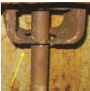
Corrosion and diminution of a quick acting cleat crutch and thinned down snugs
