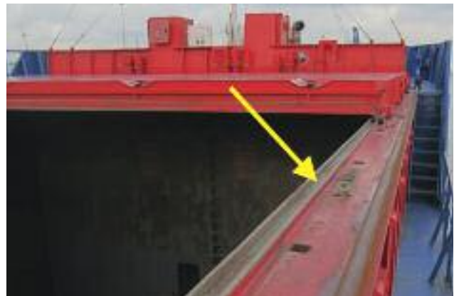
Crooked quick acting cleat (improper vertical alignment)
