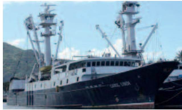
Fig 19. Large modern purse seiner showing two observation towers and two power blocks.
