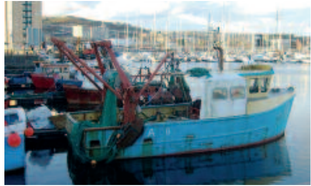
Fig 7. Typical small inshore trawler showing trawl doors hanging on aft gantry and net wound onto a net drum (UK).
