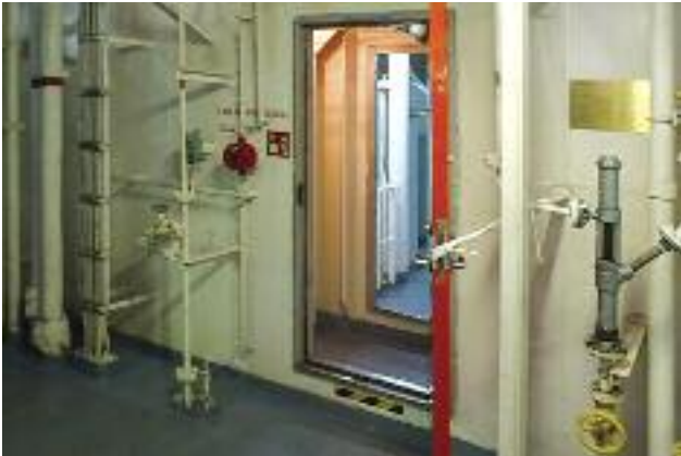
Steering gear fire doors tied open
