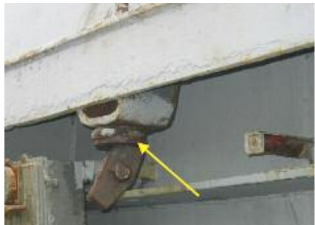
Overtightening of securing arrangements and crew member overtightening cleat with a spanner and cheater bar (top) until the rubber washer is reduced to pancake size (bottom)
