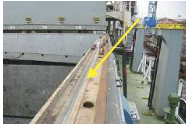
Stainless steel mating surface for sliding type packing rubber on coaming
