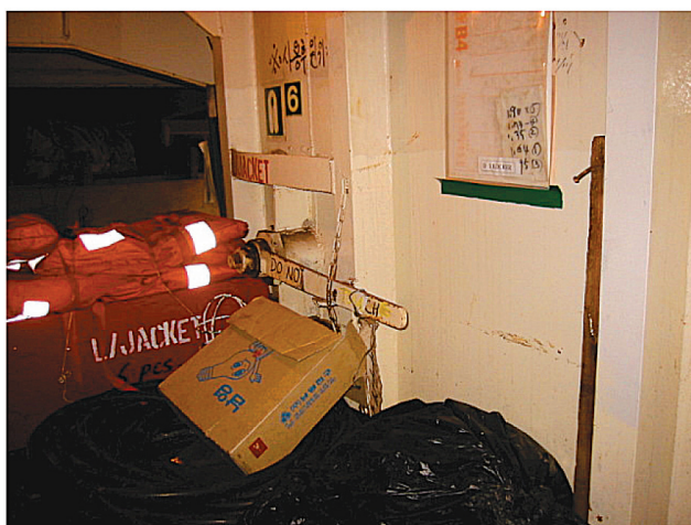
Obstructed bitter end
