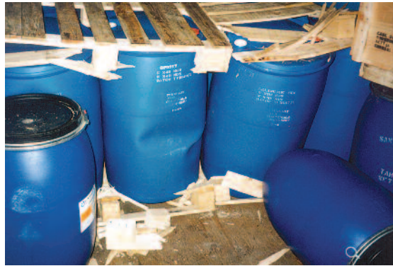
Lightweight pallets have been used for heavy cargo that has caused the pallets to break up and point packing has caused the plastic drums beneath to deform and collapse
