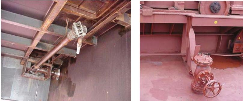
Figure 1.3: Fixed hold cleaning gun under hatch covers and fixed hold cleaning connection on deck.
