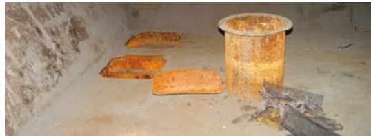
Figure 1.28: Hold suction arrangement and filter.
