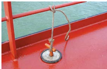
Figure 1.9: Scupper plug fitted.
