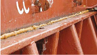
Figure 1.25: Do not use foam to seal hatches.
