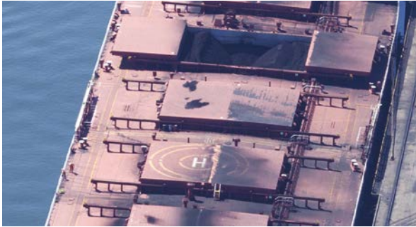
Figure 1.10: In ports where helicopters are used for pilot transfer, it is a normal requirement of the port to wash down the helicopter area and at least one hatch length either side of the helicopter area (ensuring that cargo debris is not washed into the dock).
