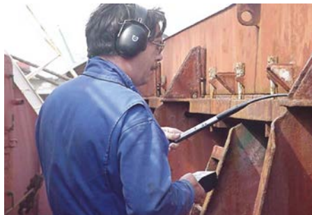
Figure 1.12: Ultrasonic hatch testing for leaks.
