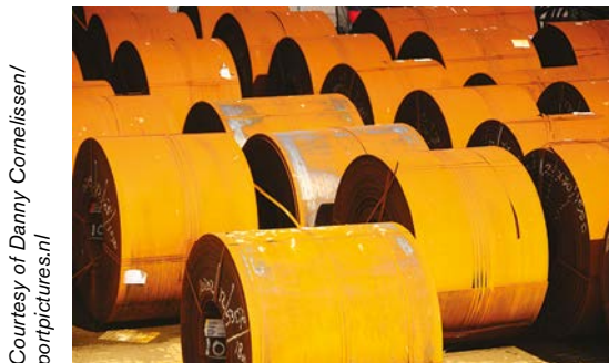
Figure 12.5: Coils showing external rust.
