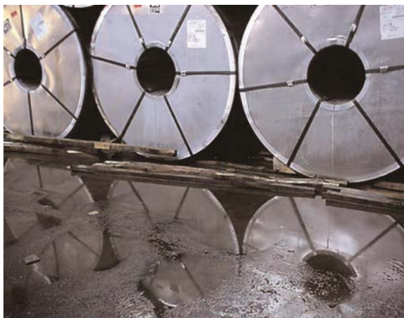
Figure 12.3: Coils of cold rolled steel.
