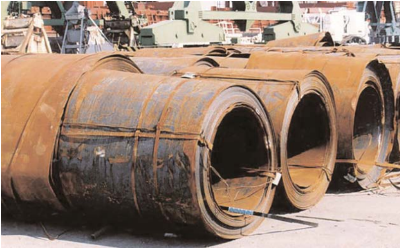
Figure 12.7: Hot rolled coils that have telescoped.
