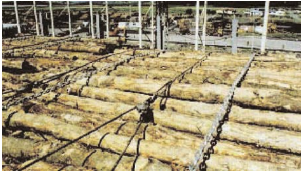
Figure 14.7: The correct use of wobble wires through snatch blocks, which are used to bind and consolidate the log stow and are independent of the number and pitch of cross lashings required. Photo shows chain cross lashings pitched 3 m apart for a stow not exceeding 4 m in height above the weather deck at the ship's side.
