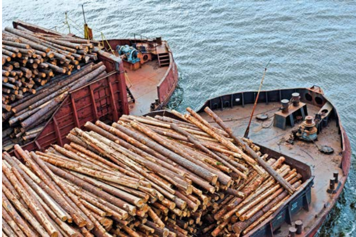
Figure 14.4: Timber cargo poorly stowed and improperly secured.
