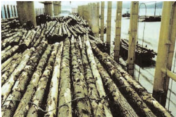
Figure 14.6: Rigging hog wires for deck-stowed log cargo, as required by the TDC Code.
