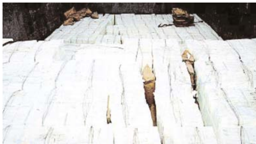
Figure 15.3: Unitised wood pulp. Note the use of airbags to secure the stow.
