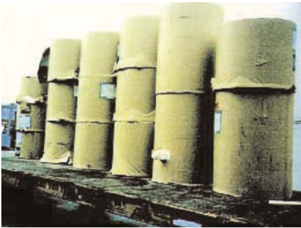
Figure 15.5: Reels of newsprint showing tears and cuts both in the wrappers and paper before shipment.
