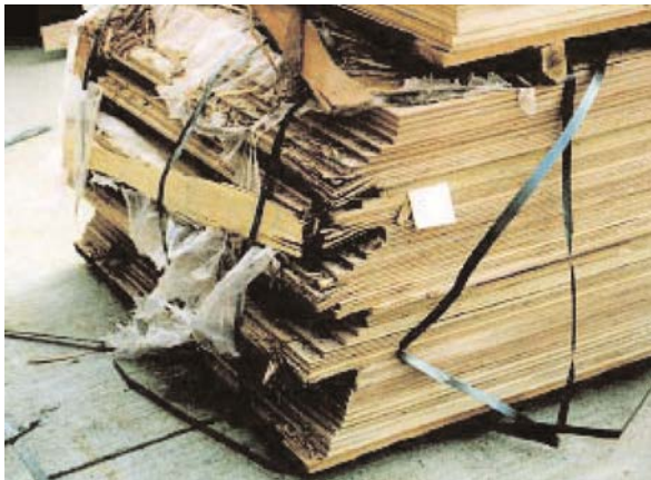
Figure 15.1: Plywood bundle showing torn plastic sheeting and loose and broken strapping bands.
