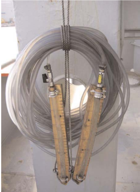
Figure 16.3: Manometer showing plastic tubing (30 to 40 m long), fitted at each end with a valve and scale. The valves are to allow the water in the tube to be retained without any air bubbles when the device is not in use.
