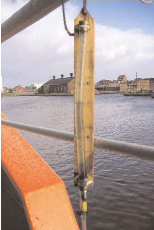
Figure 16.4: Manometer, showing scale and water level. When a scale is fitted and used for the reading, care must be taken that the scale is fixed at the same height on each side of the vessel.
