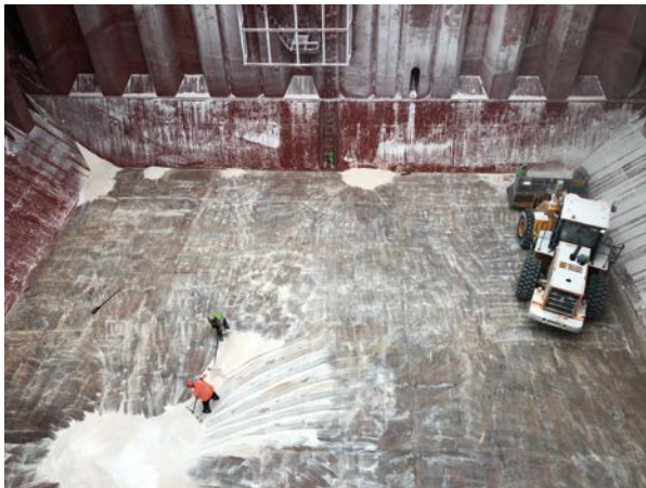
Figure 17.2: The exact type of hold cleaning will be determined by the requirements of the cargo for safe carriage and to prevent taint/spoilage/damage.
