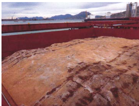
Figure 2.6: Surface damage to cargo as a result of ship's sweat.
