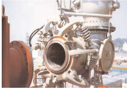
Figure 23.7: MLA quick connect/disconnect coupler (QC/DC).
