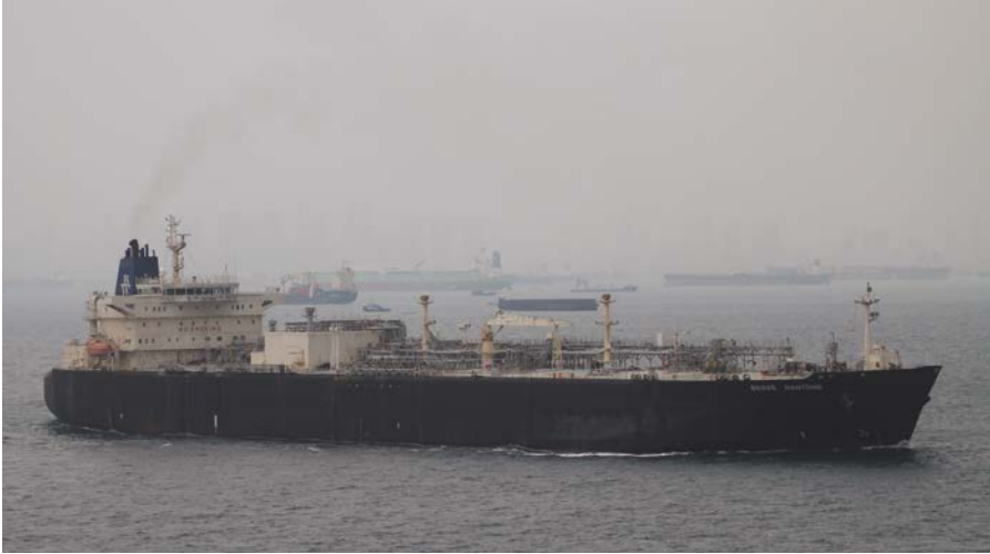
Figure 23.4: Fully refrigerated LPGC.
