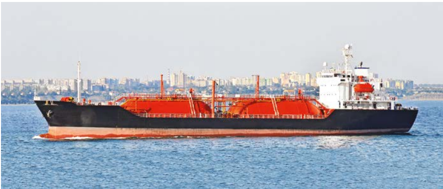
Figure 23.2: Pressurised LPGC with cylindrical tanks.
