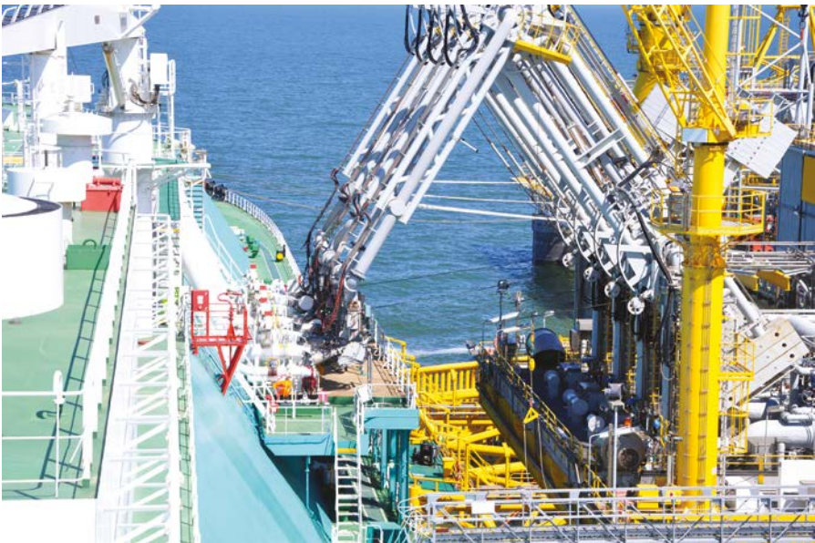
Figure 23.6: MLAs at cargo manifold (on an LNGC).
