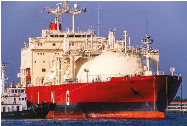
Figure 24.1: LNGC with Type B tanks (Kvaerner Moss system).
