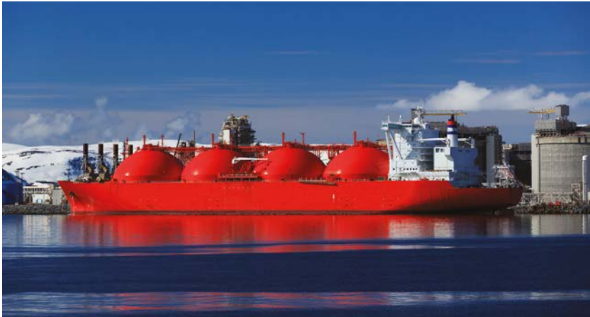
Figure 24.3: LNGC with Type B tanks (Kvaerner Moss system).
