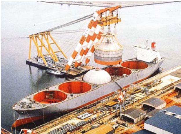
Figure 24.8: LNGC with Moss (spherical) tanks.
