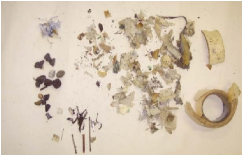
Figure 24.4: Debris recovered from the ship's manifold strainers after loading a commissioning cargo at a new LNG export terminal.
