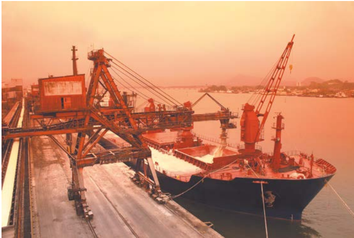
Figure 25.2: Raw sugar in Santos, Brazil, being loaded as a bulk cargo directly into the cargo holds.
