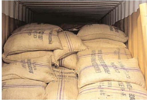
Figure 27.2: Container lined with kraft paper.
