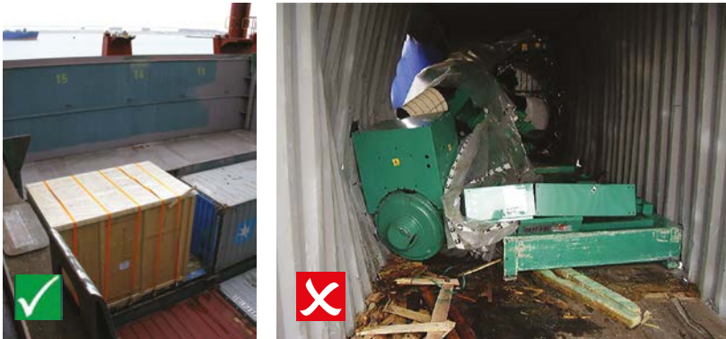
Figure 45.15: Cargoes should be well packed and properly secured inside CTUs. Failure to do so can lead to extensive damage to the CTU, surrounding cargo and even the ship itself.
