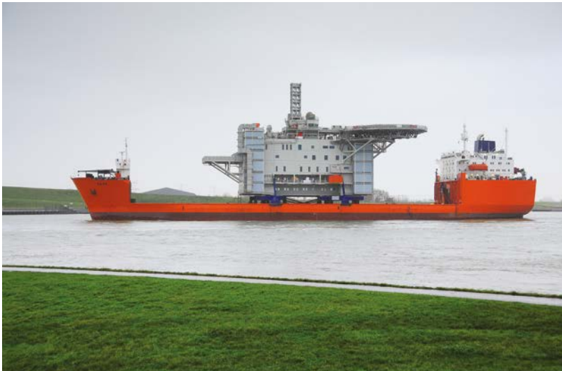
Figure 45.28: A float on/off vessel with an offshore platform as its cargo.
