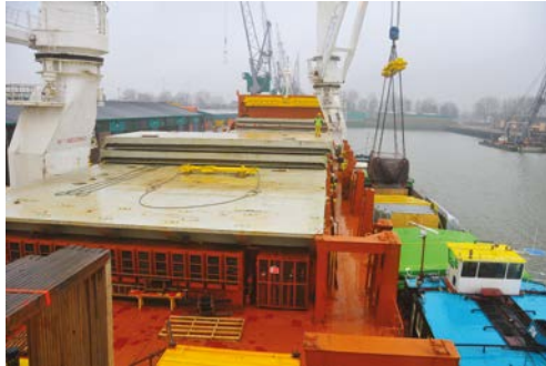
Figure 45.10: Loading heavy-lift cargo on to an inland barge.
