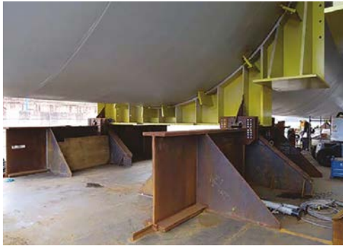
Figure 45.38: Where cargo units may incur deflections due to the longitudinal bending of the vessel, the sea fastenings must be carefully designed to minimise the loads imparted into the cargo unit. More complex sea fastening designs are required, based on specialist expertise. It is, therefore, important that sufficient time is allowed in the project for the proper design process to be carried out.
