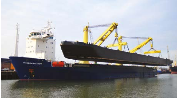
Figure 45.25: Cargo being unloaded using a tandem lift.
