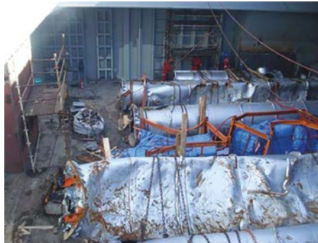
Figure 45.2: Damage to project cargo during transportation.
