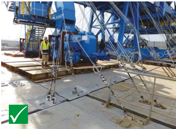
Figure 45.22: Lashing wires with sufficient scope and clear working space.
