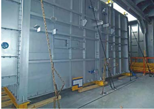
Figure 45.35: Lashing chains need to be properly tensioned and so need to be secured to appropriate securing points to enable the tension to be created. The chains shown provide good tipping restraint but minimal sliding restraint, due to their high angle.
