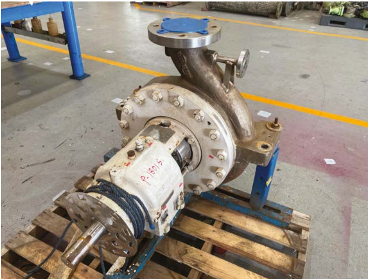
Figure 48.4: Engine spares and equipment are regularly stored and transported on pallets. These can be hard to rig and lift due to the centre of gravity (CG) of the item being unknown.
