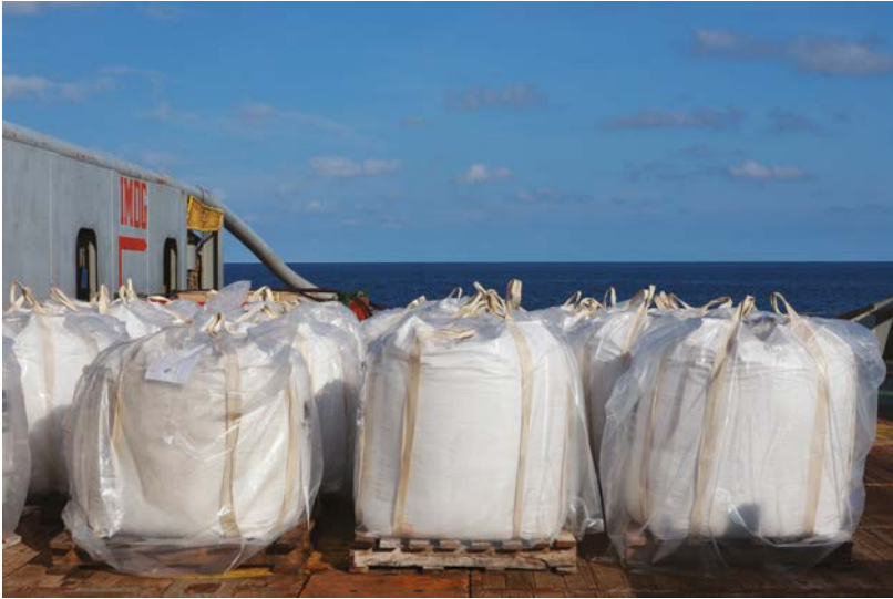
Figure 48.1: Example of best practice when transporting palletised items by sea. The contents of the heavy duty bag do not overhang the pallet, they are wrapped in plastic to avoid weather damage or items spilling, and the item is secured to the pallet with plastic strapping. The ship's crane can then lift the heavy duty bag/pallet by its lifting strops.
