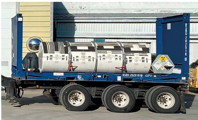
Figure 49.2: UF_6 cylinder being loaded onto a flat-rack container.
