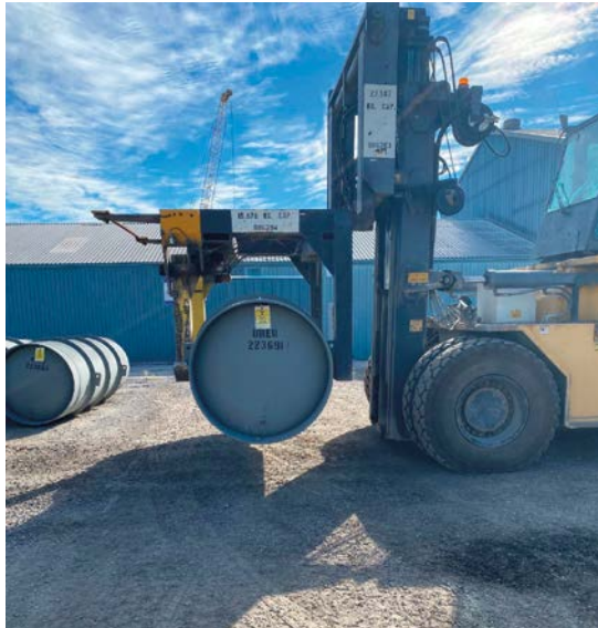
Figure 49.3: 48 inch cylinder for natural UF_6 .
