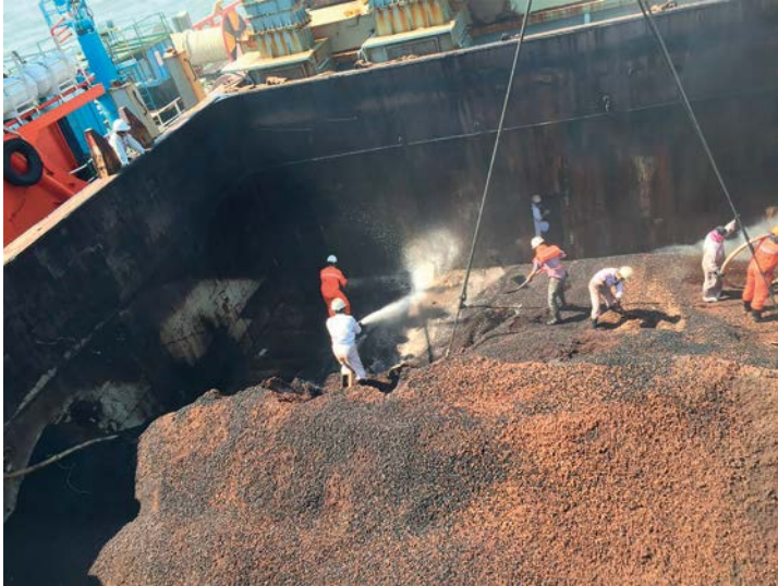
Figure 50.3: Heated and discoloured seed cake cargo (corn gluten feed).
