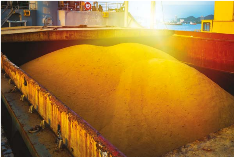
Figure 51.1: Bulk cargo loaded in a heap in the centre of the hold.
