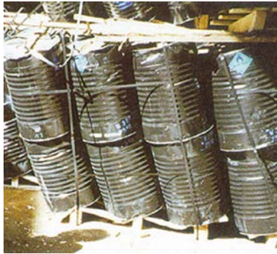
Figure 53.3: Heavy drums that have broken loose from inadequate strapping.
