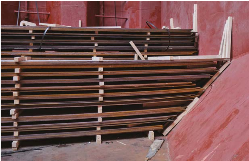
Figure 53.2: An example of timber dunnaging for steel plates.
