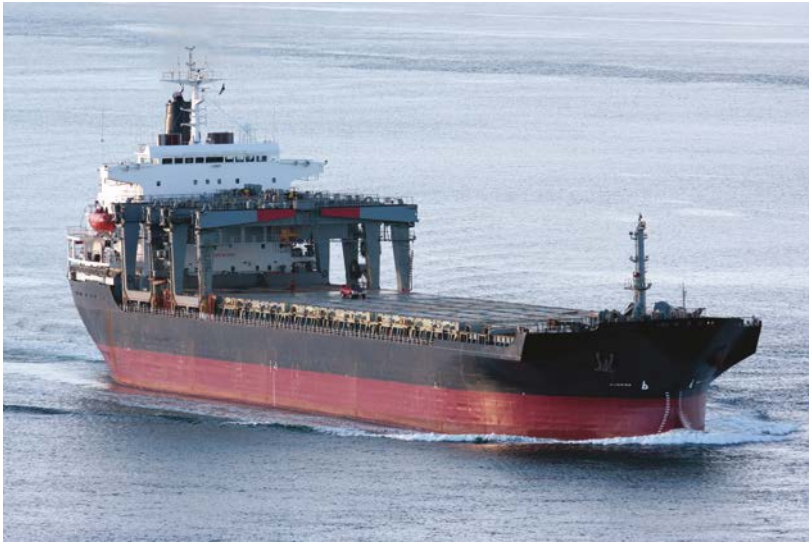
Figure 53.1: Medium-sized bulk carriers often replace tweendeckers on trades that have not been containerised or where, because of the type of cargo, it is impossible to use containers.
