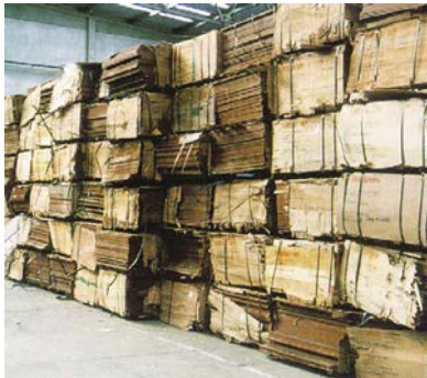
Figure 53.4: Plywood bundles that have broken out of packing that is insufficient for the weight of the bundles and bearers.
