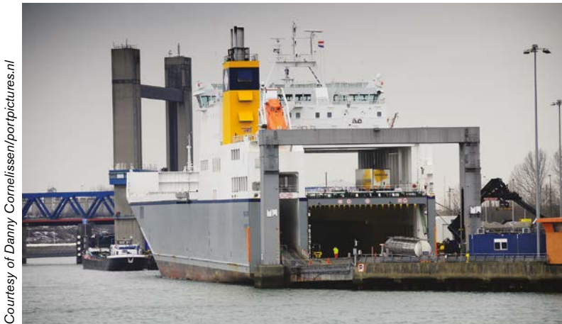
Figure 54.1: Many areas above the actual hold space on RoRo vessels can reasonably be considered as 'on deck' even though they are not fully exposed to the onslaught of wind and sea.
