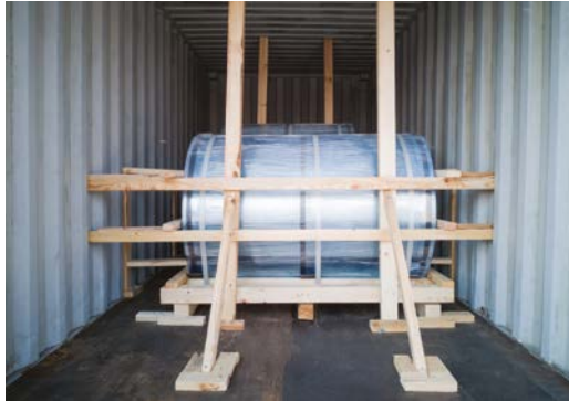
Figure 54.2: An example of best practice when securing cargo within a container.
