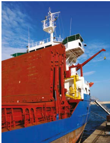
Figure 55.1: Steel hatch covers.
