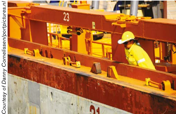
Figure 55.6: Hatch coaming and cleat arrangement on a container ship fitted with pontoons.
