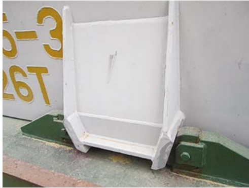
Figure 55.13: Properly maintained and adjusted locator.
