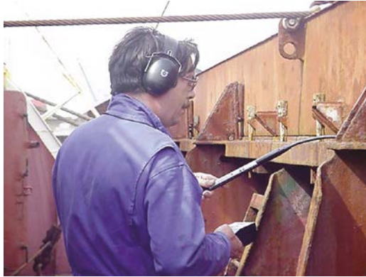
Figure 55.19: Ultrasonic testing of hatch cover.
