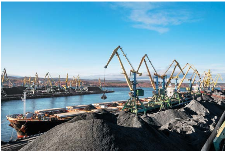
Figure 6.1: Where coal cargoes are subject to rainfall in the load port, they should be covered where possible but always reinspected and retested to confirm their moisture level.
