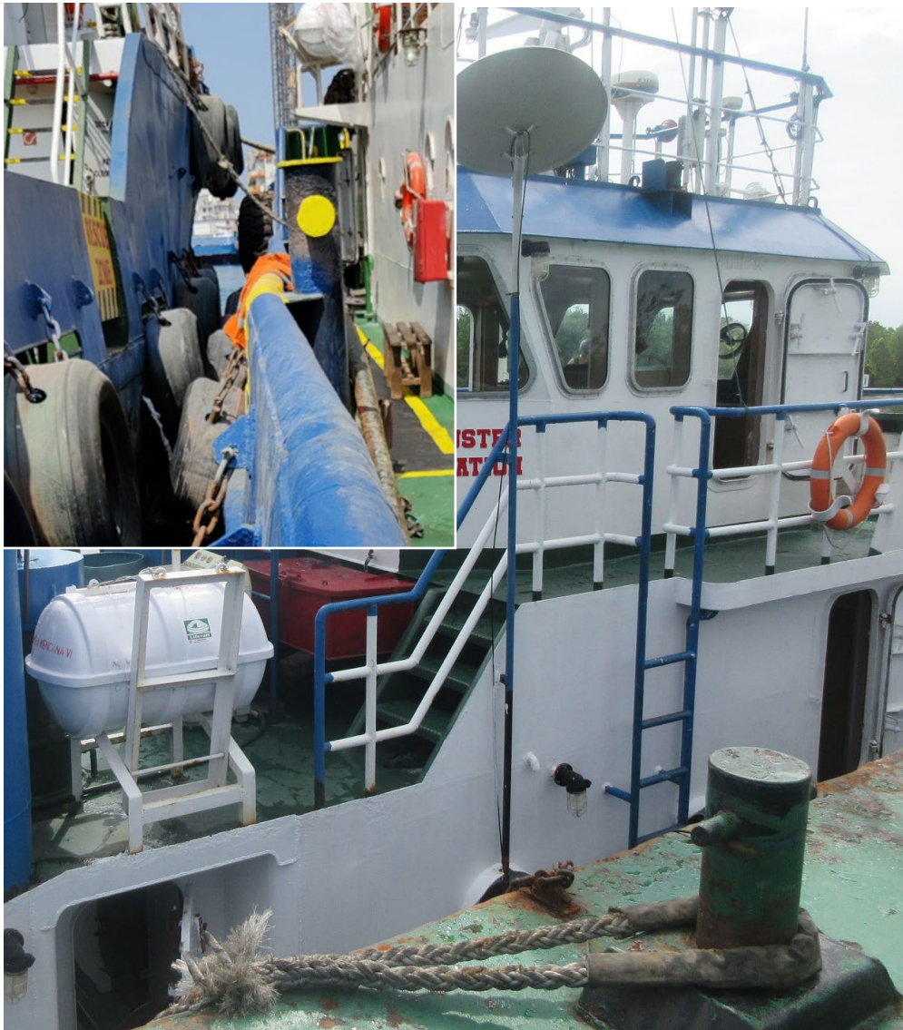
X No means of safe access has been provided.
