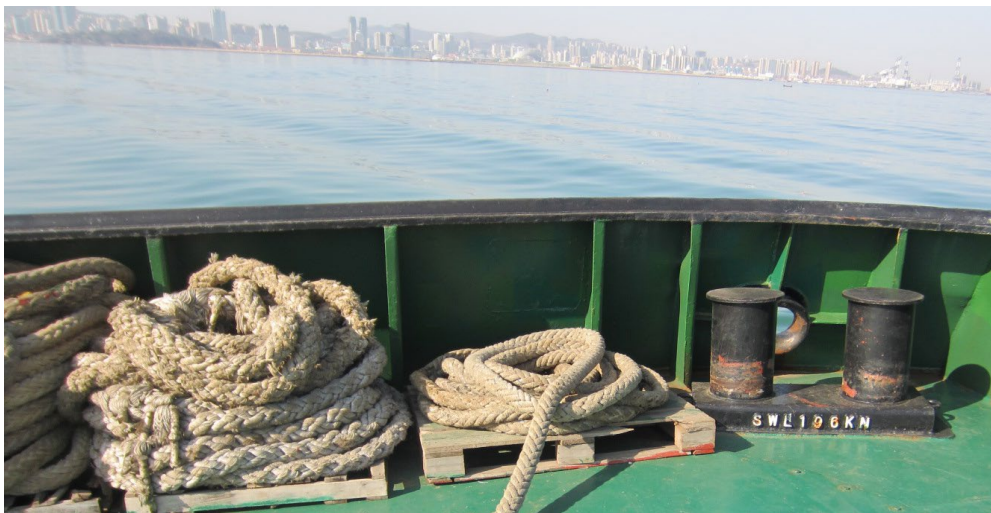
X Ropes stowed off deck but not protected from sun and weather.
