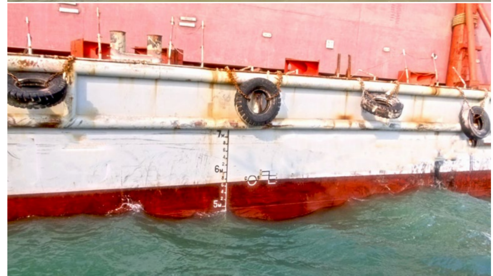
Vessel and barge draught marks and water in void space.
