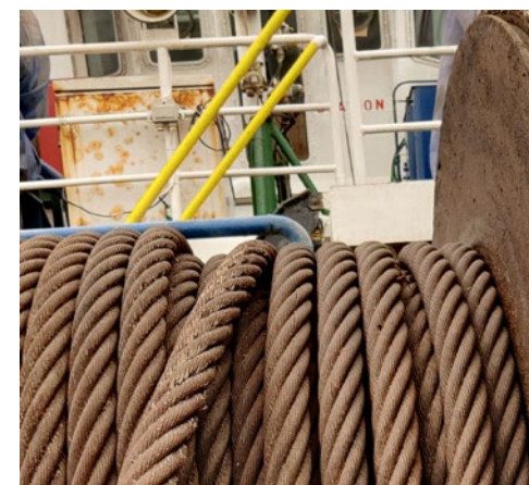
X Wire ropes should be routinely inspected and greased as applicable.
