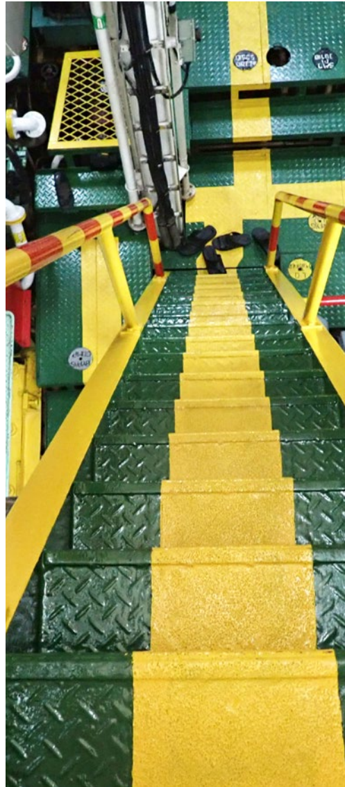
✓ Safe walkways and good highlighting of changes in deck level and permanent trip hazards
