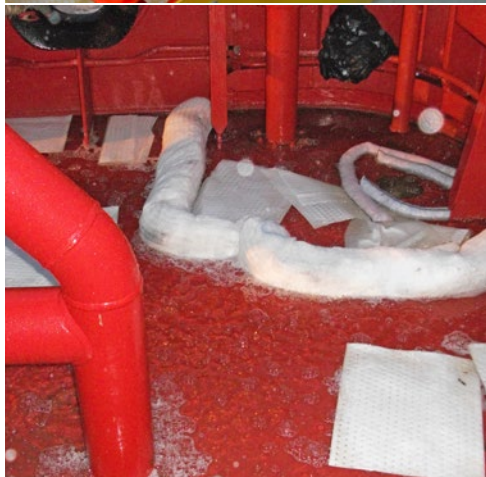
✓ Adequate SOPEP equipment readily available on deck.
