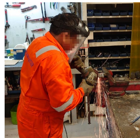
✓ Safety guard fitted on angle grinder and face shield and gloves in use.
