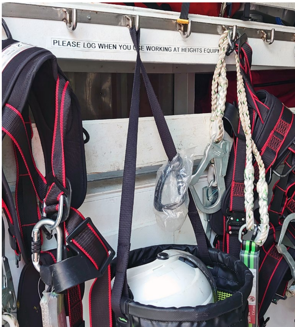
✓ A WaH locker containing a range of personal fall prevention equipment, including full body harnesses in a range of sizes.
