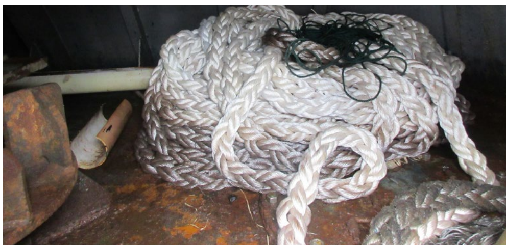
X This rope is soaking up oil from the deck. Oil, paints and other chemical contaminants may degrade the fibre ropes.
