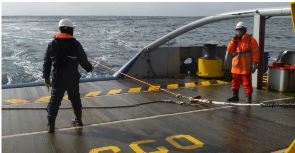
✓ PPE lines marked on deck. Lifejackets required when working close to the open stern.
