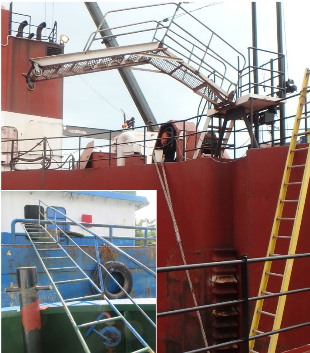
X If a portable ladder is used, it should be in good condition, secured and used with caution.
