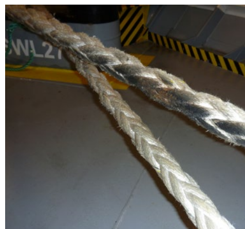
X Ropes allowed to be squeezed between the tug and barge will suffer damage.
