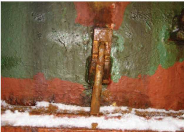
Crooked quick acting cleat (improper vertical alignment)
