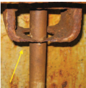
Corrosion and diminution of a quick acting cleat crutch and thinned down snugs
