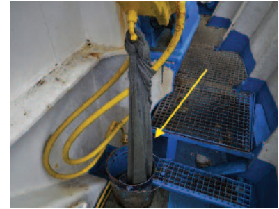
Temporary repair (rubber patch and jubilee clip) and shipboard made systems to contain hydraulic oil leakage from hydraulic piping and cylinders
