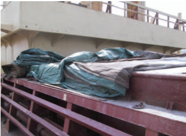
Different plies of tarpaulins used for making hatch covers weathertight
