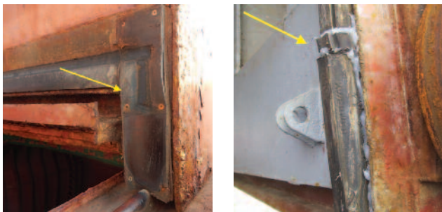
Backing strips (here nailed into the original packing rubber) and short insert repairs are frequently seen as evidence of improper repairs
