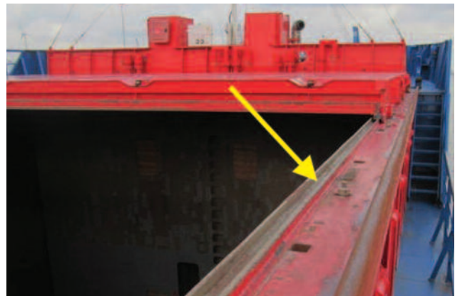
Crooked quick acting cleat (improper vertical alignment)
