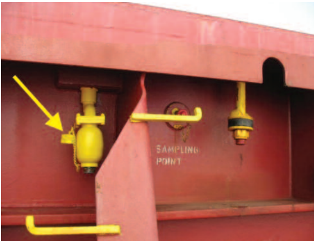
Drain valve (yellow) with threaded fire cap firmly connected by a lanyard
