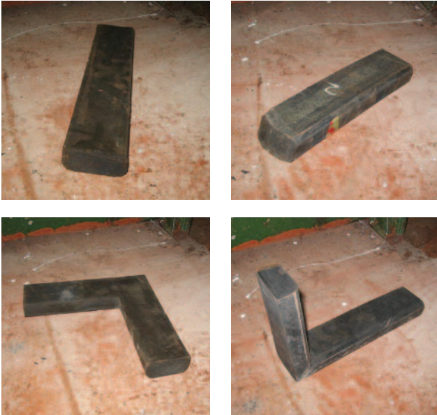
Different shapes of packing rubbers (from left to right: linear rubber, end piece with solid nosing, flat corner and vertical corner)
