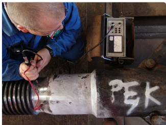
Non-destructive examination of a hook
